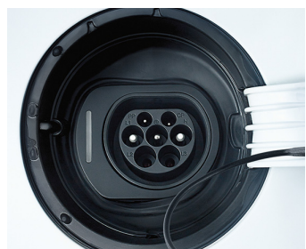
AC charging socket
